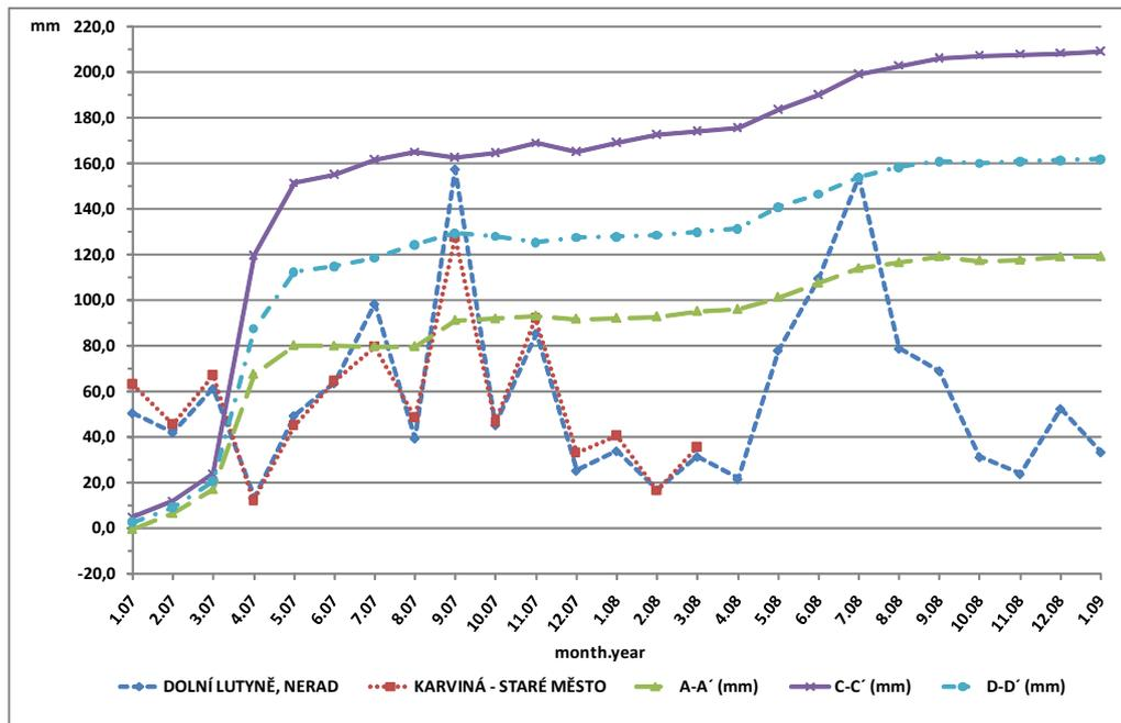
Fig. 4. Chart of measured landslide movements and monthly precipitation from two nearest rainfall gauging stations to the Doubrava Oplíží slope deformation for the monitored period
