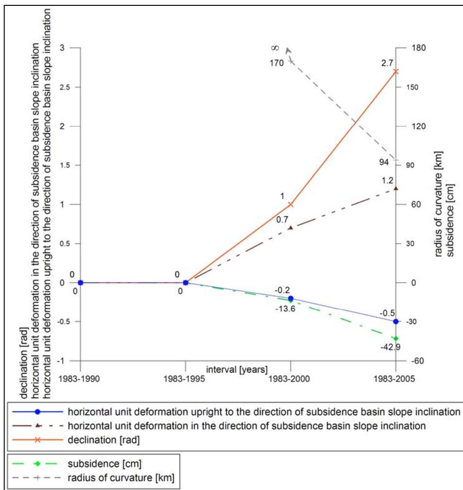
Fig. 3. Chart of terrain deformation parameter changes on the Doubrava Oplíží slope deformation during the monitored time periods
