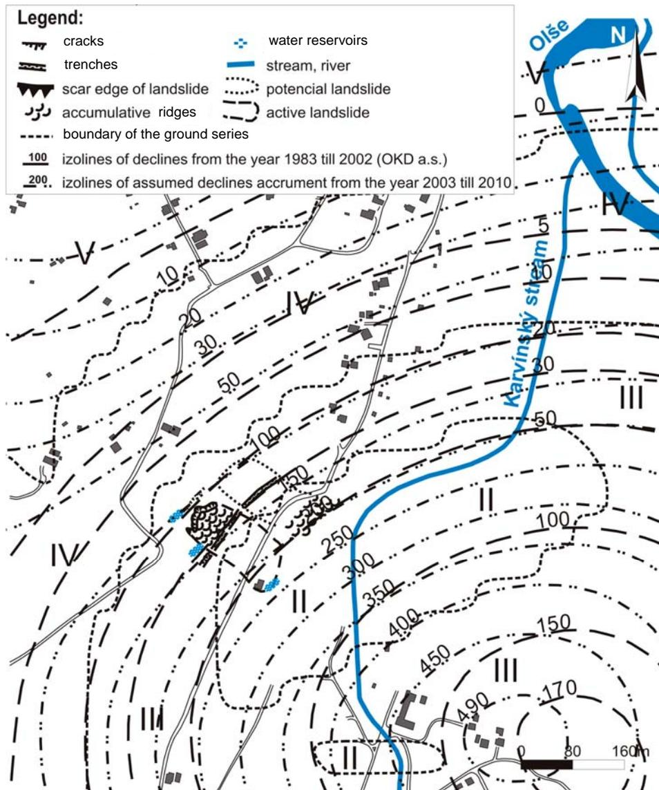
Fig. 2. Declines in centimetres caused by mining in the periods of 1983–2002 and the forecast increase by 2010 with marked positions of slope deformations
