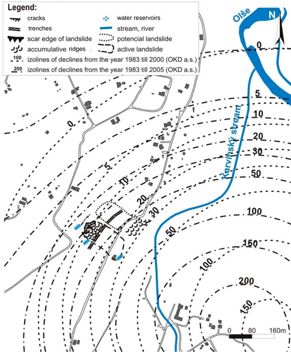
Fig. 1. Declines in centimetres caused by mining in the periods of 1983–2000 and 1983–2005 with marked positions of slope deformations
