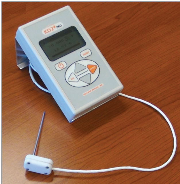
Fig. 1. KD2Pro thermal conductivity meter and TR-1 sensor
