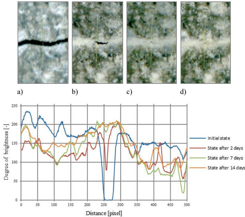
Fig. 5. Image of the sample surface with a crack and an intersection line: (a) immediately after cracking, (b) after 2, (c) 7 and (d) 14 days of self-healing and graphs of the brightness degree along the intersection line
